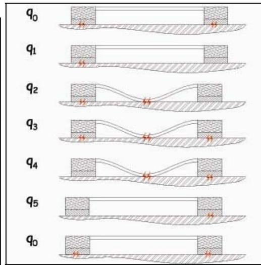
**Figure 2:** Step sequence of the  $\mu$ Walker.
