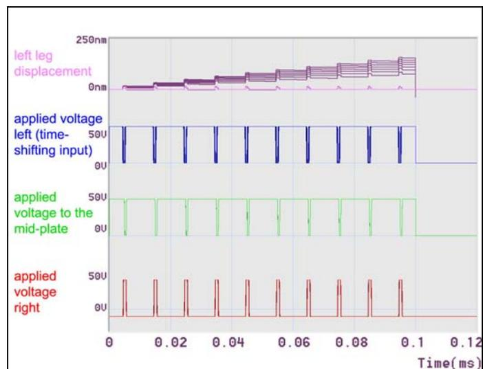
**Figure 6:** Time-shifting of the input 'applied voltage left' is here used for step size control.
