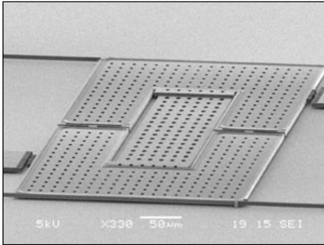
**Figure 1:** 1D-version of the  $\mu$ Walker used for modeling.
