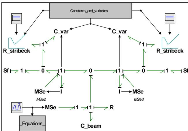
**Figure 3:** 20-SIM model of the  $\mu$ Walker.
