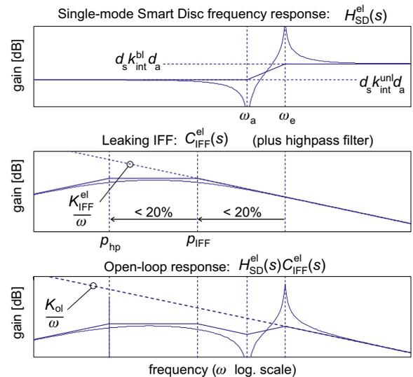
Fig. 2. IFF-controller design, based on the Smart Disc frequency response.
