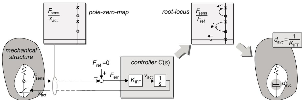
Fig. 1. The Smart Disc frequency response, from position actuator to collocated force sensor, is characterised by an alternating pole-zero-pattern. Upon application of Integral Force Feedback, all resonances are damped (poles moving into the left half of the  $s$ -plane). The Smart Disc then effectively behaves as a viscous damper.
