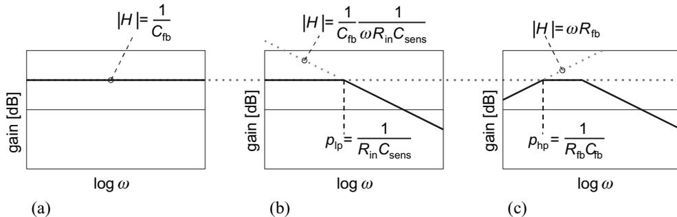
Fig. 4 Frequency response functions (asymptotic approximation) corresponding to the electric circuits in Fig. 3.
