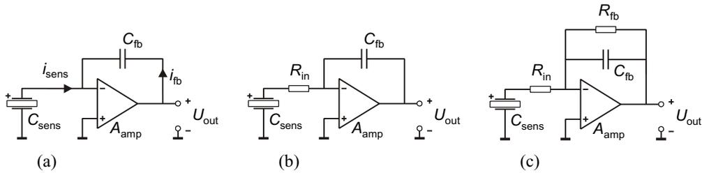
Fig. 3 (a) Basic scheme of a charge amplifier, (b) extended with first-order lowpass behaviour, (c) extended with first-order highpass behaviour. (Remark: the '+' indicates the positive electrode of the sensor.)
