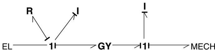
Fig. 7. Bond graph of Fig. 6 enhanced with causal strokes.
