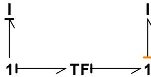
Figure 56: Dependent inertia's via de causal constraints of 1-junctions and transformer (cf. Figure 14)
