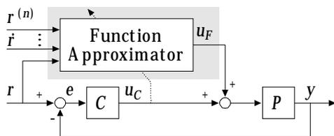
Figure 1: Originally proposed Feedback Error Learning controller
