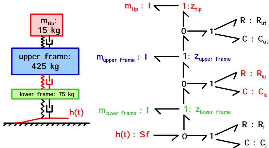
Figure 3. Iconic diagram and bondgraph of a mobile robot
