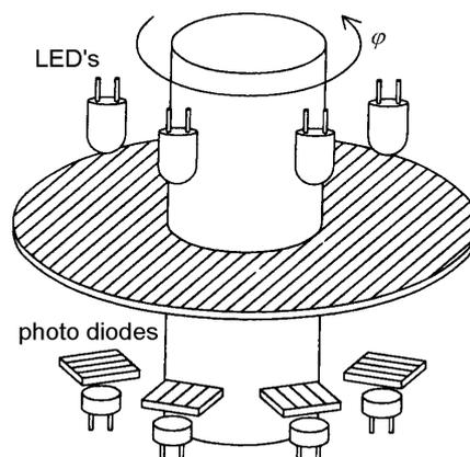
Figure 6. The rotational sensor
