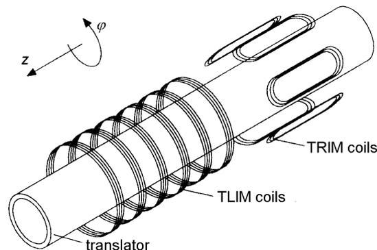
Figure 5. The windings for the Translational motor (TLIM coils) and for the Rotational Motor (TRIM coils)
