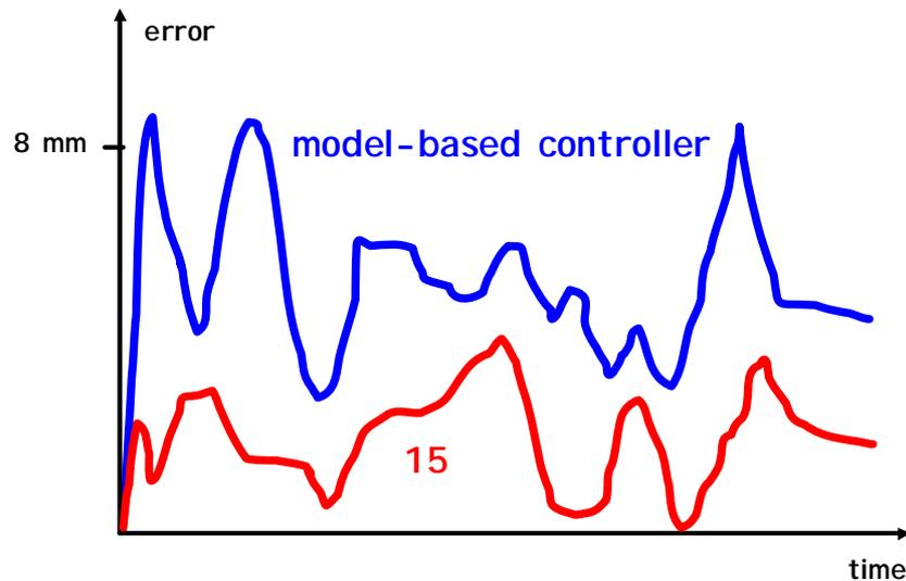
Figure 13. Comparison of a learning feedforward controller and a model based controller
