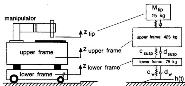
Figure 10. Model to determine the weight distribution over the upper and lower frame
