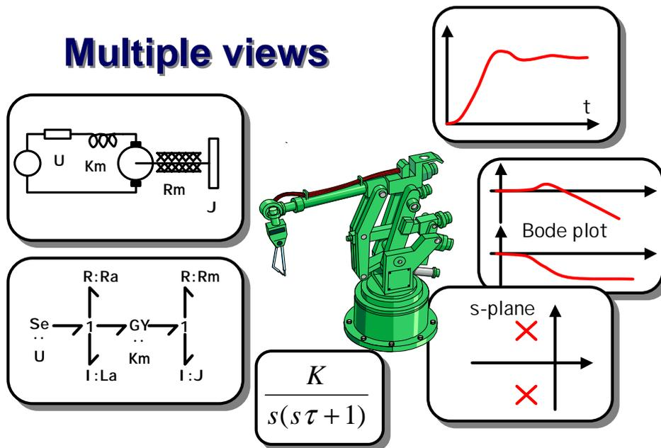
Figure 4. Multiple views of a servo system in open loop and closed loop
