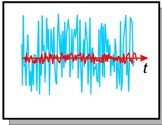
Figure 8. Error signal before training the network (about  $\pm 100\mu\text{m}$ ) and after ten standard motion patterns (about  $\pm 5\mu\text{m}$ )
