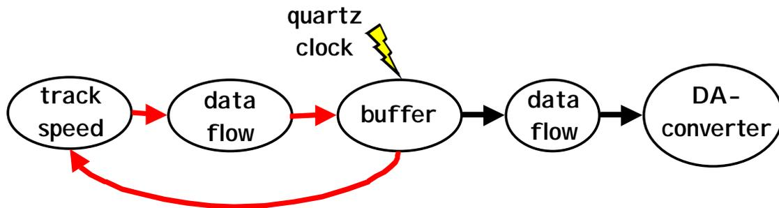
Figure 2. Combination of closed-loop and open-loop control in a CD-player
