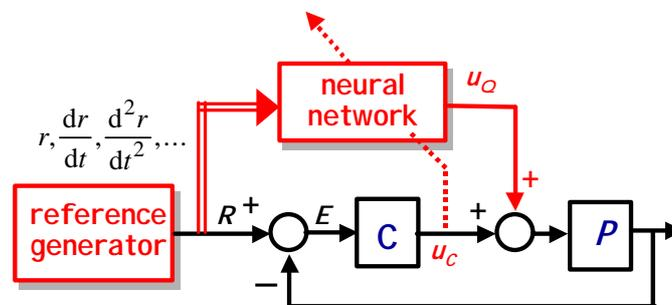
Figure 7. Learning feedforward control. The neural network is trained by the output of the feedback controller
