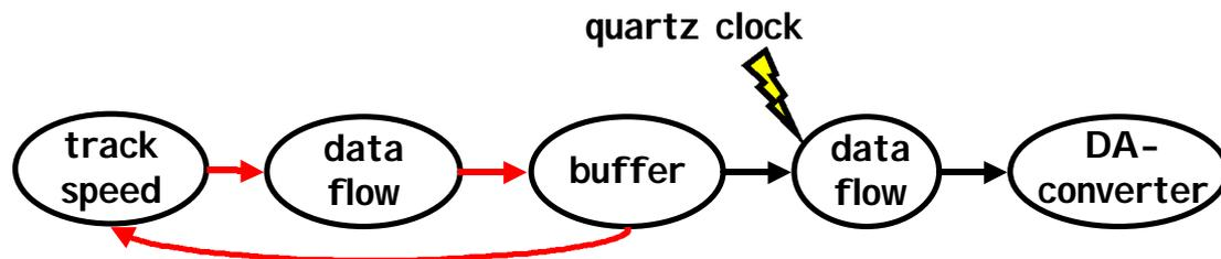
Figure 1. Combination of closed-loop and open-loop control in a CD-player
