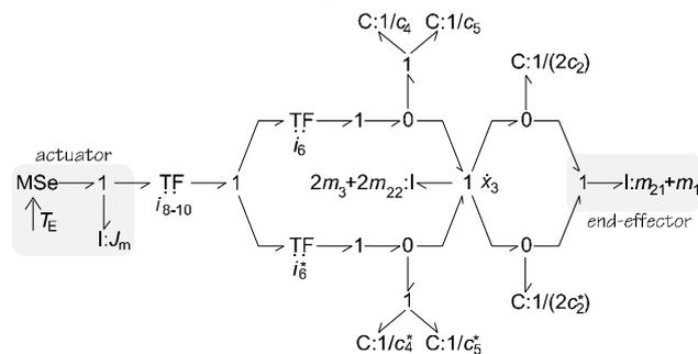
Figure 3: Initial bond graph model of A0-plotter
