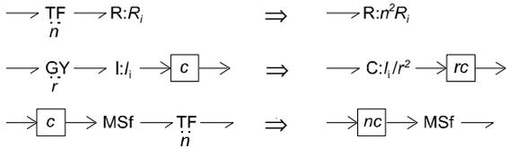
Figure 5: Composition of a transmission and an element
