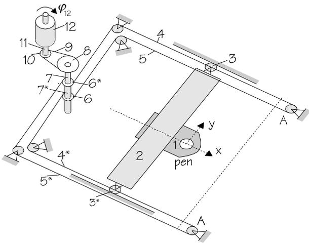
Figure 2: Sketch of the A0-plotter to be designed
