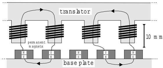
Fig. 3 Magnets of the linear motor
