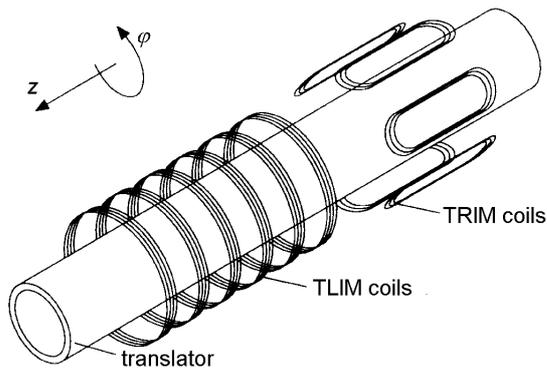
Fig. 2 The windings for the Translational motor (TLIM coils) and for the Rotational Motor (TRIM coils)
