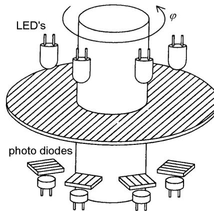
Fig. 1 The rotational sensor
