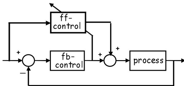
Fig. 5 Learning feedforward control. The output of the feedback controller is used as training signal for the feedforward controller
