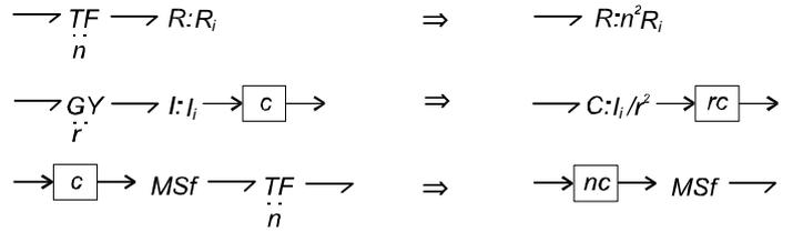
Fig. 2. Composition of a transmission and an element
