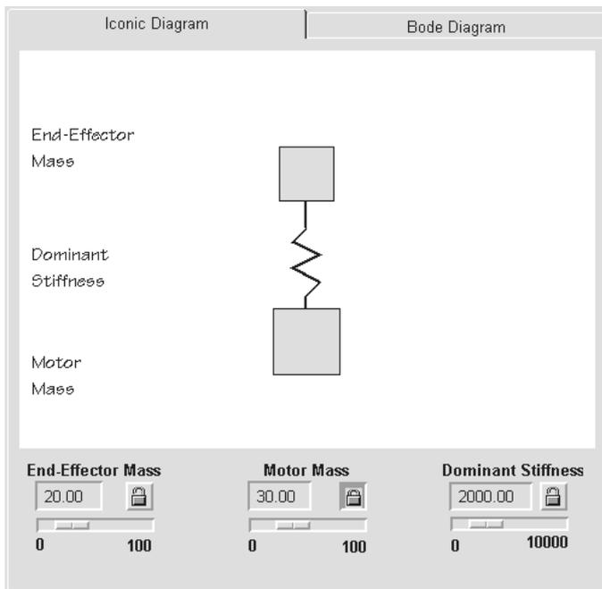
Fig. 7. Iconic diagram with variables
