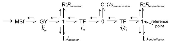
Fig. 4. Determination of direction of propagation
