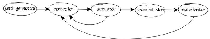
Fig. 1. Controlled electro-mechanical system
