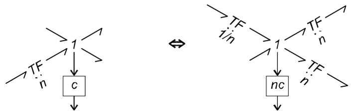
Fig. 3. Propagation of a transformer
