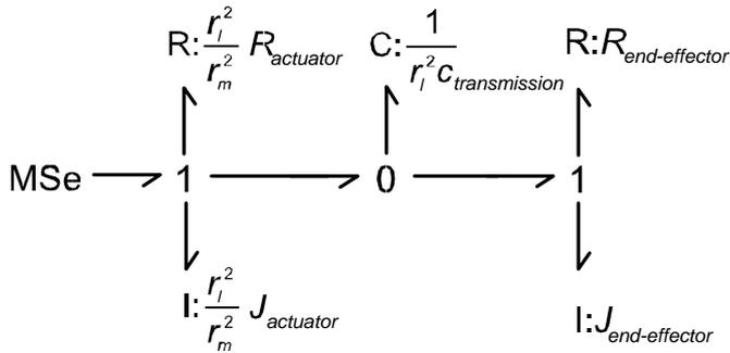
Fig. 5. Simplified bond graph model (without transformation factors)
