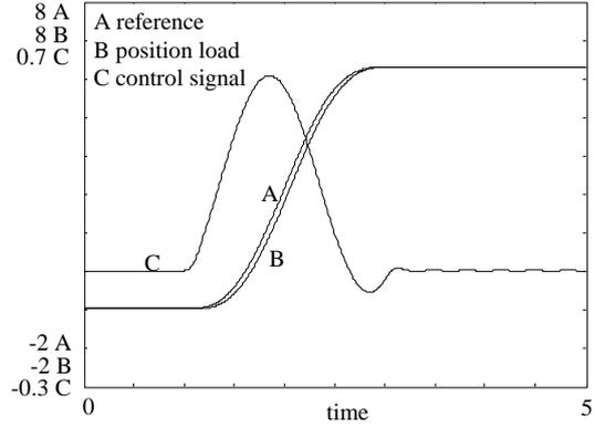
Fig. 6. Simulated response of LQR controlled system.
