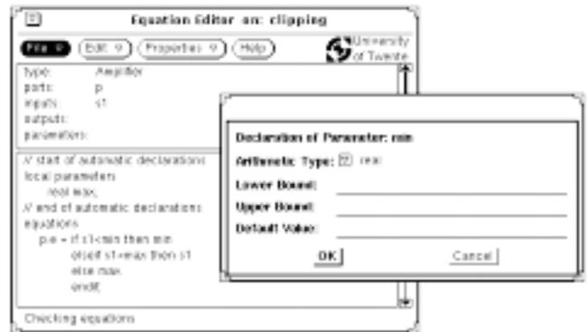
Figure 13: Equation Editor with the model for the amplifier
