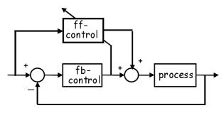
Fig. 5 Learning feedforward control. The output of the feedback controller is used as training signal for the feedforward controller
