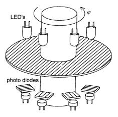
Fig. 1 The rotational sensor
